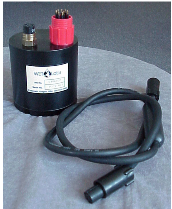
Submersible unit with patch cable
